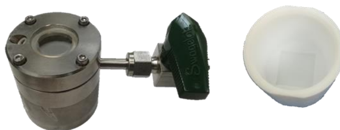
Fig. S1. Laser lithography chamber made from stainless steel with a PTFE insert and a quartz glass window.
