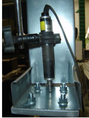
Figure 11: Screw connection LVDT's position
