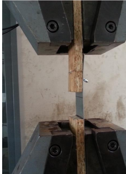
Figure 26: Experimental deformation of the OSB-to-steel screw connection
