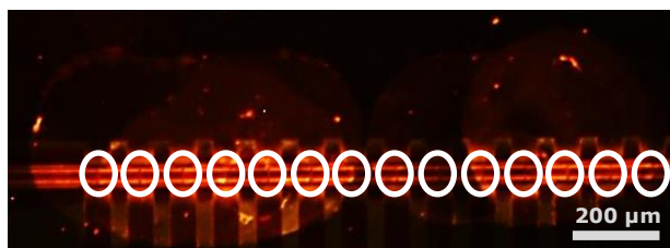
Figure 38: Fluorescence reference control of DNA immobilization on SiNW FET.
