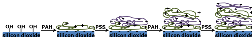
Figure 15: Schematic diagram of the assembly of polyelectrolyte multilayers.
