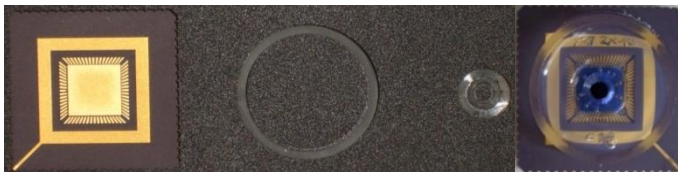
Figure 13: From individual components to the encapsulated nanowire chip.
