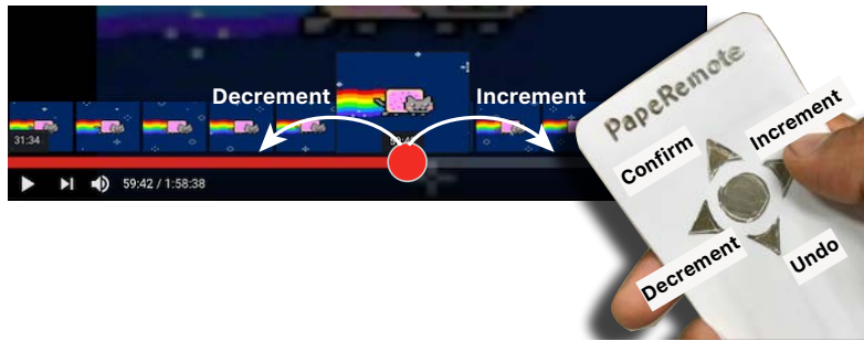
Figure 5.4: BinPut can be used to quickly and accurately scroll through a continuous range of values, for example, to navigate to an exact timestamp in a video using a DIY paper remote control made using conductive inkjet printing.
