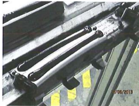
Fig 3: Example of a manually glued reinforcement plate. The applied glue stripes are not uniformly distributed along the plate.
