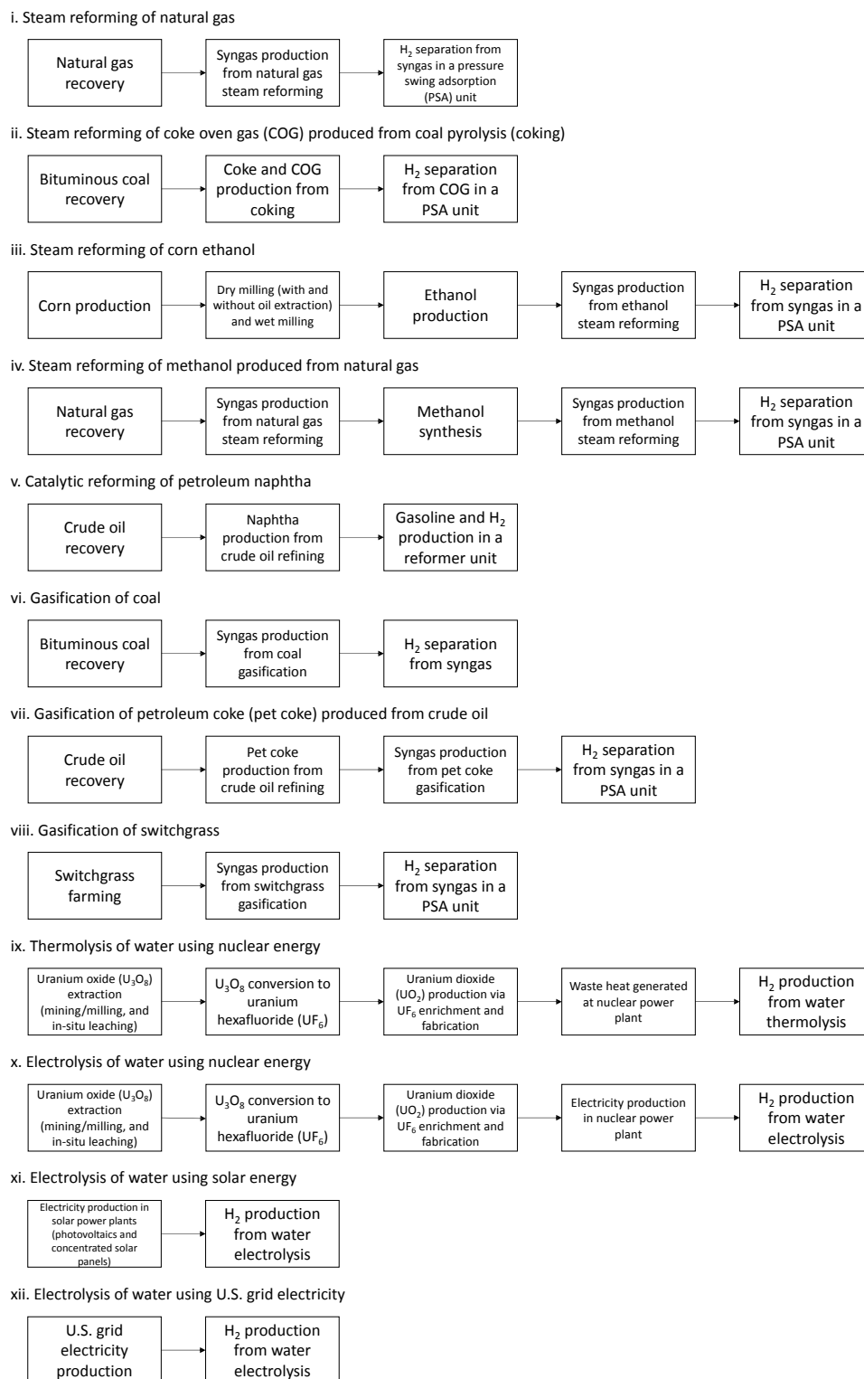
Figure S1. Process overview of the 12 hydrogen pathways employed in the lifecycle analysis calculations. Note that many lifecycle steps have been omitted for simplicity (e.g. transportation steps, water gas shift reaction, etc.).
