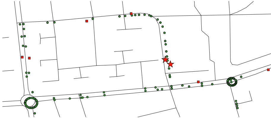
Figure 1: Israel, Kiryat Gat: example of inaccuracy. Shapes (green circles) and bus stops (red squares/stars) in GTFS displayed on an OSM network. The stops represented by the red stars show the wrong side of the road problem . Note the missing roundabout at the right side and the positional errors.
