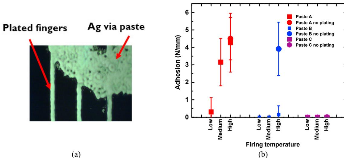
Fig. 5. (a) Optical microscope image of continuous front plated finger around Ag via paste (b) Adhesion of different Ag via paste as a function of the peak firing temperature after plating, only paste A passes the test with adhesion above 1 N/mm after plating
