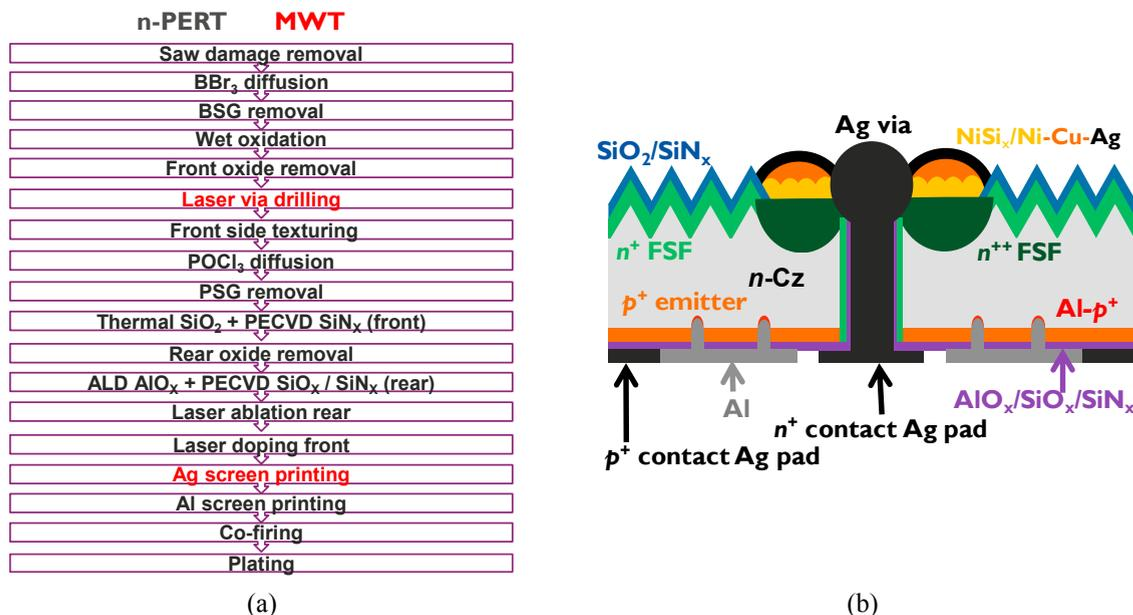
Fig. 2. (a) Process flow and (b) cell structure for our MWT PERT solar cells
