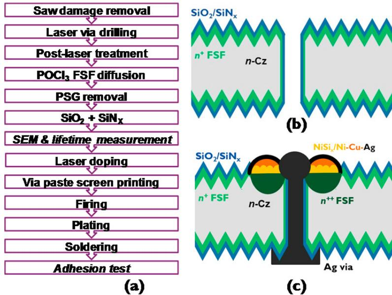
Fig. 1. (a) Processing flow for short loop tests and the structures of the test samples for the study of (b) via passivation and (c) compatible metallisation
