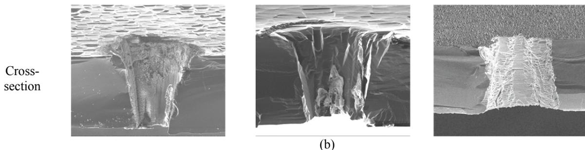
Fig. 3. (a) Top view and (b) cross-sectional SEM of the via surface after different post-laser treatments
