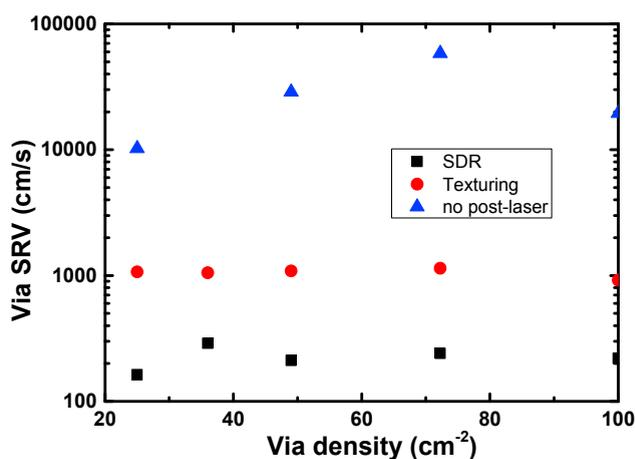
Fig. 4. Calculated via SRV after different post-laser treatments using the Mingirulli's approach [4]. The via SRV is reduced from 10000 cm/s without any post-laser etching to 1000 cm/s with KOH texturing and reduced to 200 cm/s with KOH SDR
