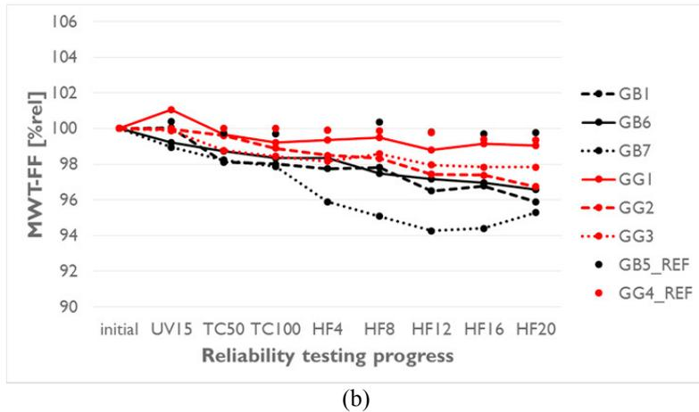
Fig. 6. Relative performance degradation of (a)  $P_{mpp}$  and (b)  $FF$  throughout reliability testing of the fabricated laminates
