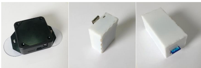
Figure 2: modules to locate multiple persons: anchor (left), tag (middle), mastertag (right)
