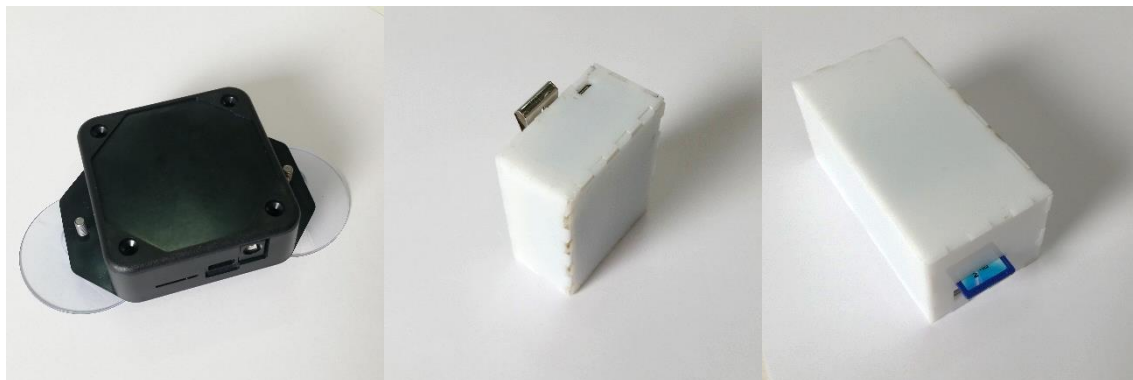
Figure 3: modules to locate multiple persons. Anchor (left) with a fixed and know position, tag (middle) which has to be worned by the residents, mastertag (right) which manages the tags and gathers the location of the residents on SD.
