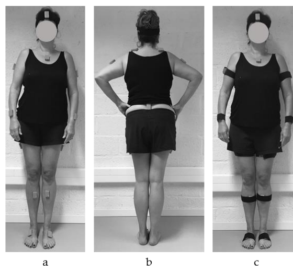
Figure 1. Inertial sensor position in (a) anterior and (b) posterior view without straps, and (c) anterior view with straps to preload the inertial sensor and minimize soft tissue artefacts.
