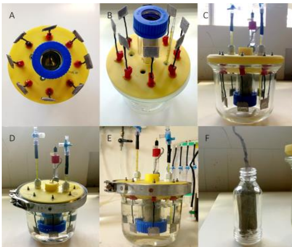
Figure 22 Set-up 8-electrode BES reactor (CMET, Ghent University, design by Dr. Kun Guo) A + B : Reversed top part of reactor, with connected WEs and CE. C : Reactor with one counter electrode (CE), eight working electrodes (WEs) and one reference electrode (RE). D : Sealed reactor, filled with 20mM acetate FWM. E : Medium is flushed with N 2 /CO 2 mixture. F : Counter electrode (CE): glass bottle filled with SS mesh as a cathode.
