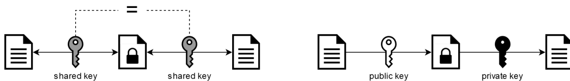
Figure 2.1: A schematic overview of how a symmetric key algorithm (left) and an asymmetric key algorithm (right) work. The arrows indicate the direction in which encryption and decryption are possible.
