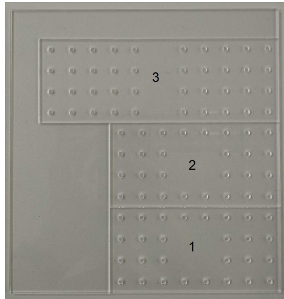
Figure 3.5: An example of the layout of a laser cut file for a model that contains three plates. The model can be seen in chapter 5.
