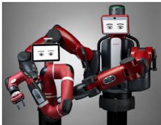
Figure 2.2: The Rethink Robotics Sawyer on the left and the Baxter on the right
