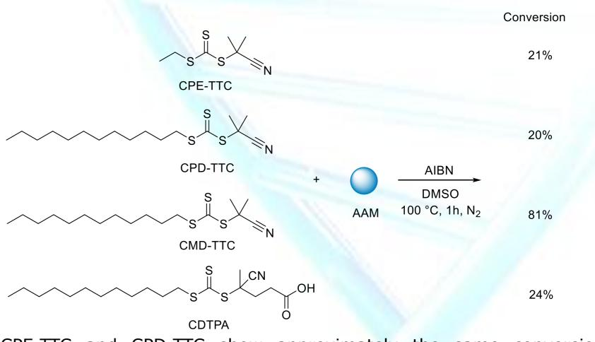
CPE-TTC and CPD-TTC show approximately the same conversion and these products are used further for the optimization of the purification process. The reactivity of CMD-TTC is too high in these conditions. CDTPA has also an interesting conversion but is unusable for purification with flash chromatography.
