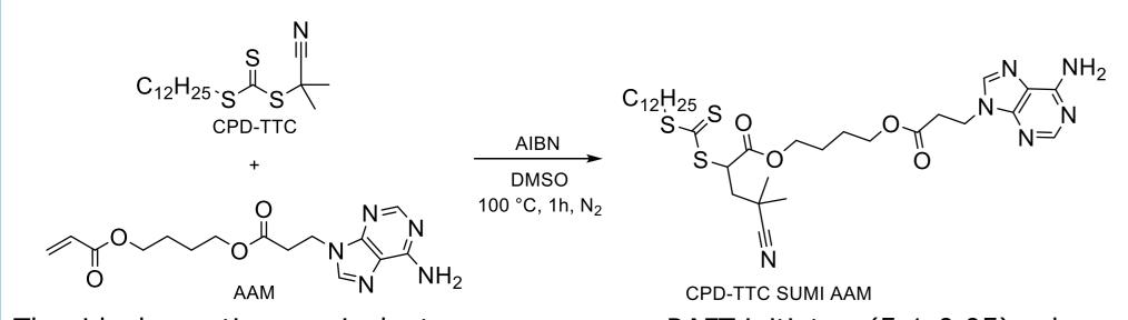
The ideal reaction equivalents are monomer: RAFT: initiator (5:1:0.05) when using AAM as monomer, CPD-TTC as RAFT agent and AIBN as initiator in DMSO when reacting 1h. at 100 °C. Purification is performed with flash chromatography when using MeOH:DCM (7:93) as mobile phase. A purity of 95% was achieved and confirmed with <sup>1</sup>H-NMR analysis
