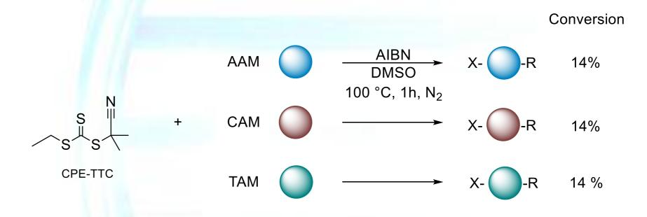
The conversion of adenine-, cytosine- and thymine acrylate monomers was tested. All three monomers showed the same conversion of 14%. Therefore, it is likely that all experiments performed with AAM would function with CAM and TAM,
