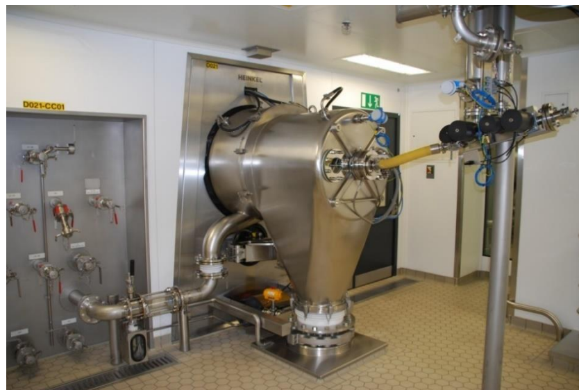
Figure 23 picture of centrifuge dryer Heinkel F3 in module B
