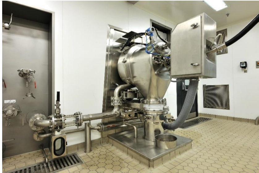
Figure 22 picture of centrifuge dryer Heinkel type F1 in module A
