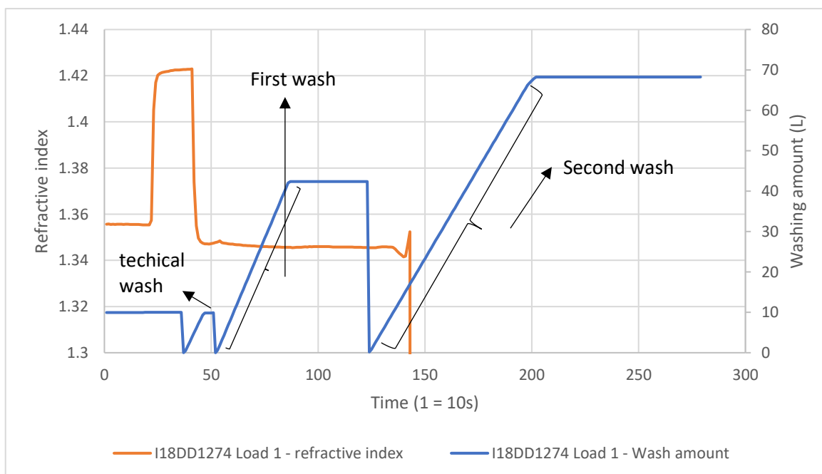
Figure 66 Alios T3730 batch I18DD1274 ideal washing curve
