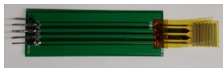
Figure 1-2 Microheater on polyimide foil
