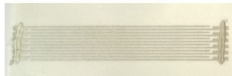
Figure 1-1 Moisture content sensor of the capacitance measuring type.
