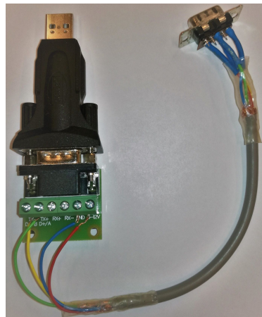
FIGURE 5.8: A Do It Yourself (DIY) USB to RS-485 adapter
