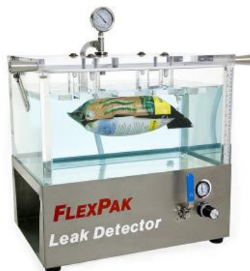
Figuur 31: Bubble test 'Leak Detector Master Easy' [67]
