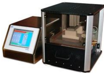
Figuur 33: Vacuum decay methode: PTI Veripac [72]
