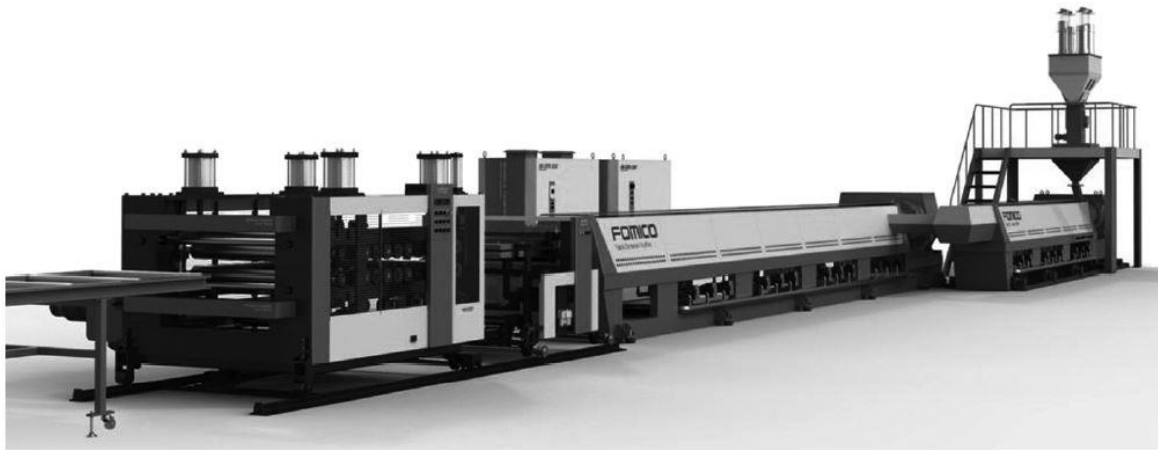
Figure 30: A photo of XPS foam production 150 mm/200 mm tandem line [22]
