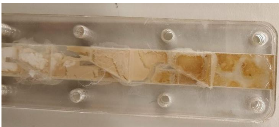
Figure 53: Crumbled, dried out structure of an output with PEO and PEO+MMT as test materials
