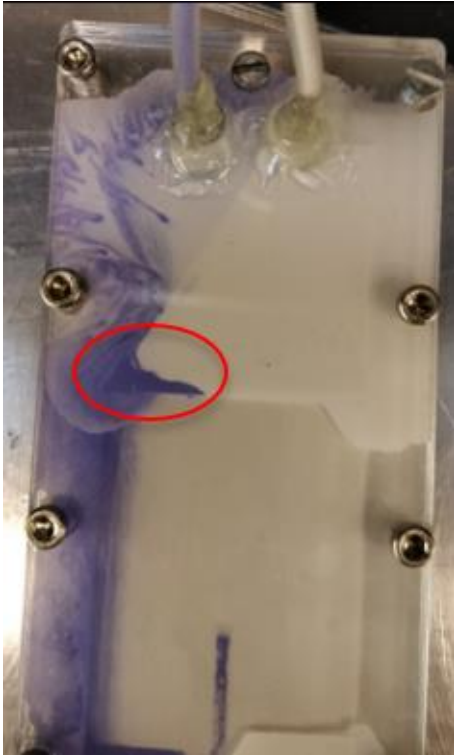
Figure 35: Result of a failed test carried out with the second version of the static mixer
