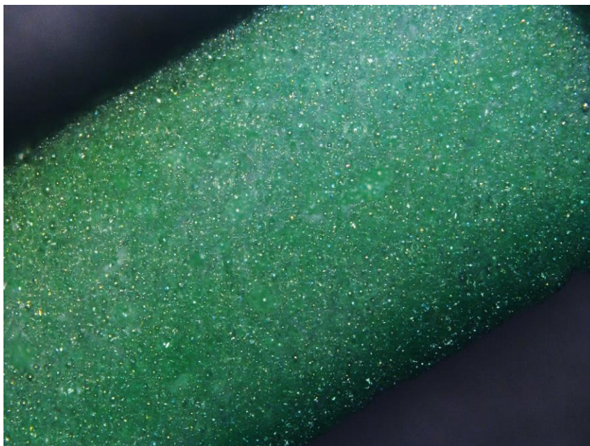
Figure 23: Microscopic view of manually created output with white and green airy clay mixtures
