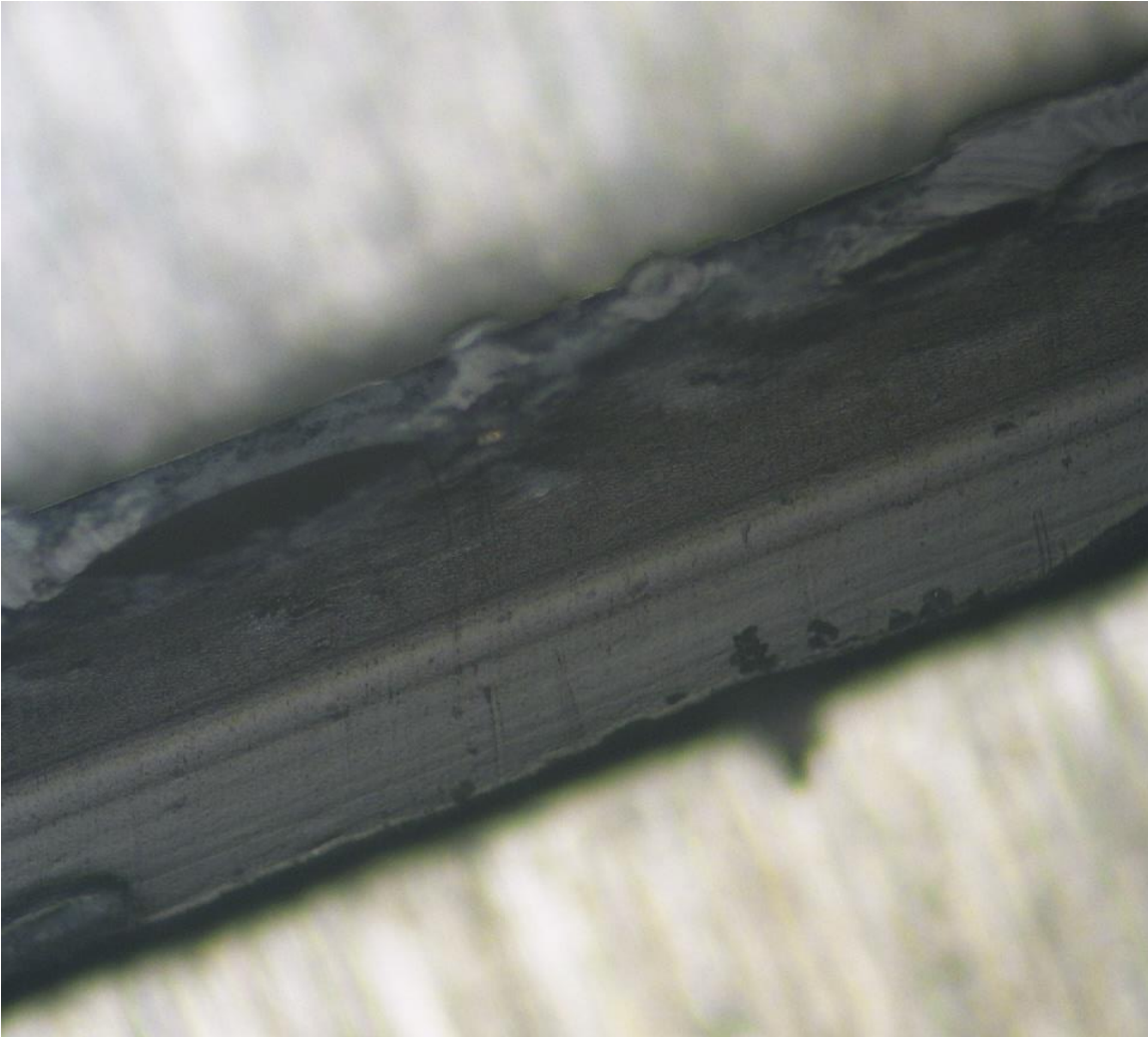
Figure 50: Microscopic view with a magnification of 5X of an output using (PEO+MMT) -suspension as test material
