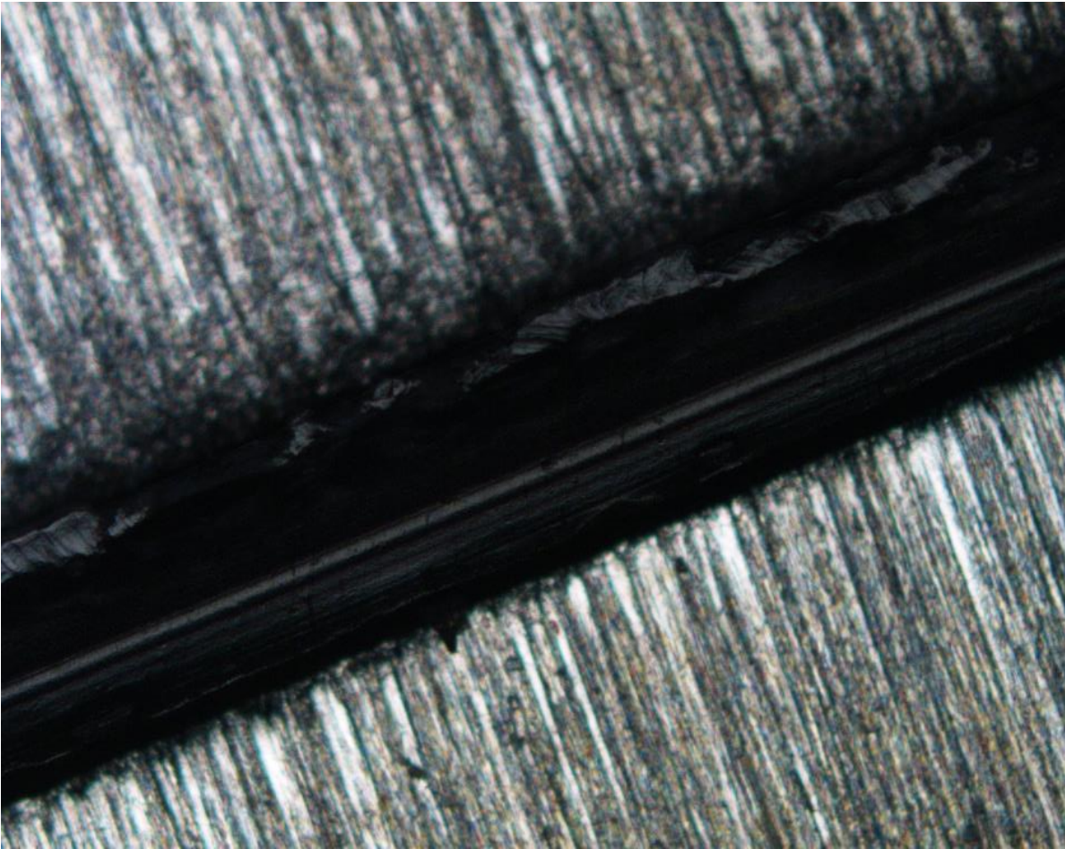
Figure 49: Microscopic view with a magnification of 5X of an output using (PEO+MMT) -suspension as test material
