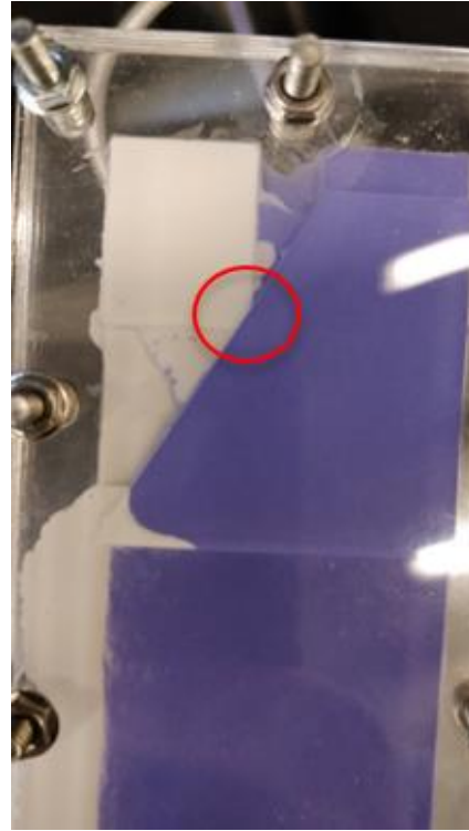
Figure 36: Result of a failed test carried out with the second version of the static mixer
