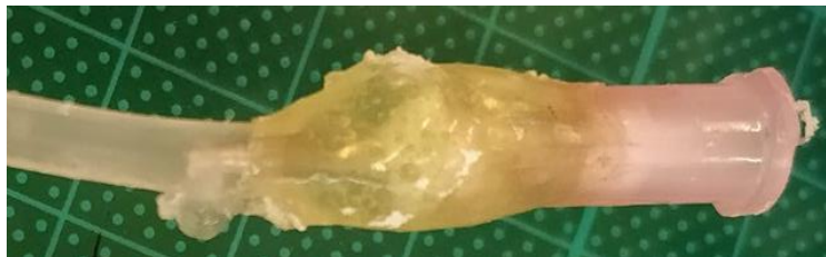
Figure 51: a leak in the glued zone
