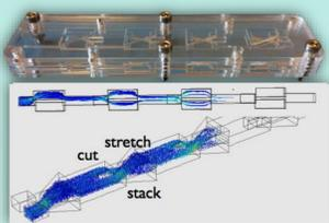
Figure 2: Flow of a material through the static mixer
