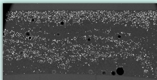
Figure 8: Output of Epofix mixtures with 6 μm PS particles and MMT particles
