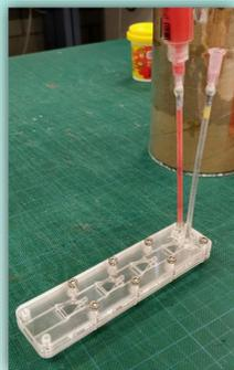
Figure 3: Static mixer setup
