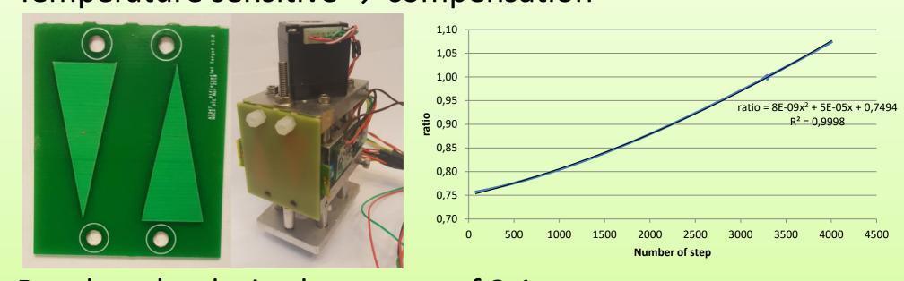
Reaches the desired accuracy of 3,1 μm
