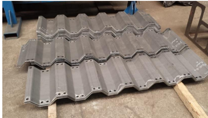
Figure 78: Initial corrugated steel plates
