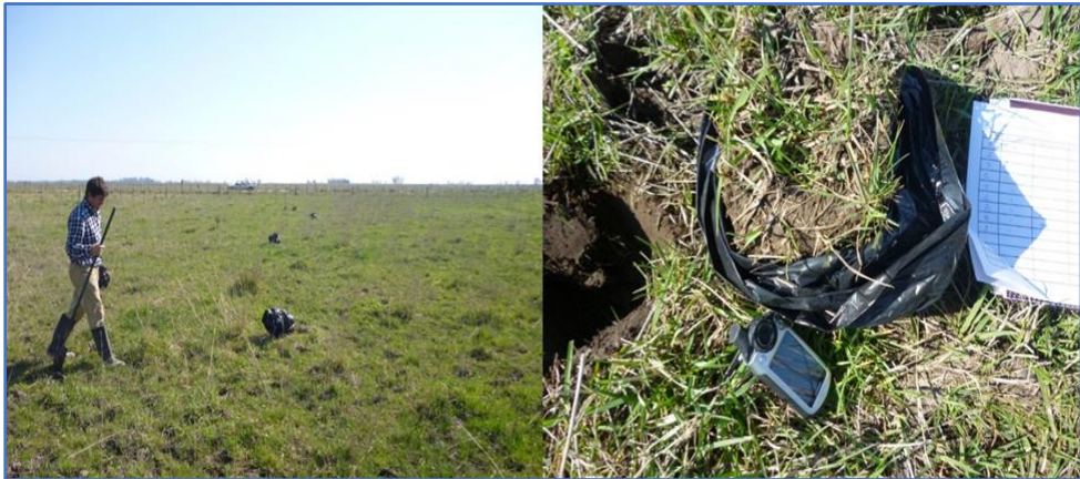
Figure 4.2. Pictures taken during sampling proceeding. On the left picture, the transect is indicated by the bags containing the samples already taken. On the right, one sample next to the record log and the GPS used to indicate de position of each single sample.
