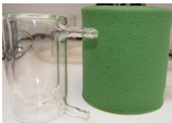
Figure 2. A homemade double walled titration vessel (left); a polyurethane jacket (right).
