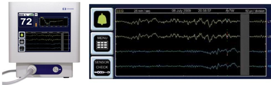
Figure 1. BIS VISTA™ monitor with EEG display. The BIS VISTA™ device is able to display bilateral frontotemporal EEG traces in real-time.
