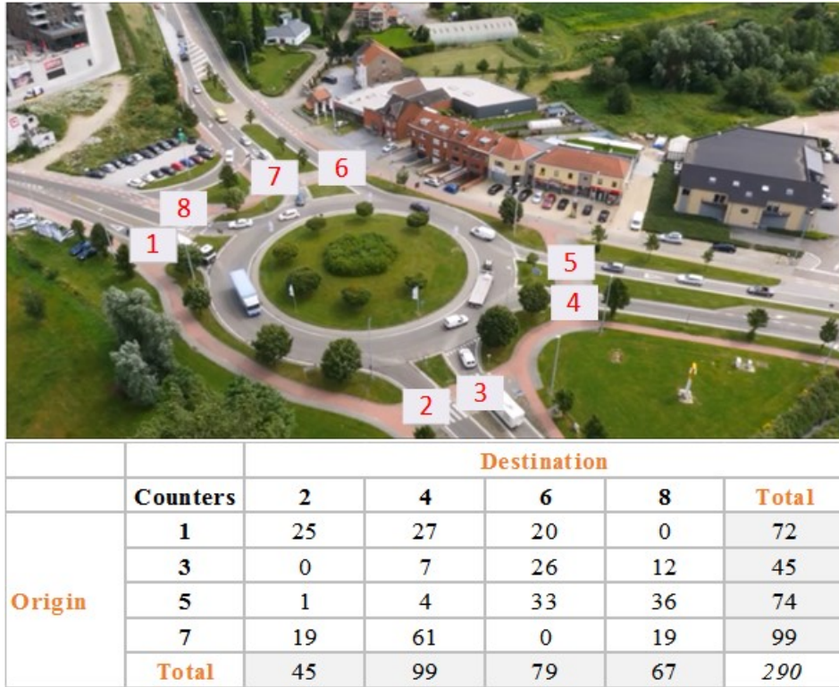
Figure 6.4: Position of virtual counters at roundabout approaches; and the Origin-Destination(OD) matrix for the roundabout traffic
