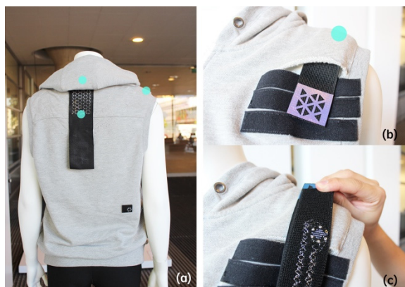
FIGURE 3. (a) Back view of the garment; (b) Adjustable design; (c) Sensor embedded in the strip.
