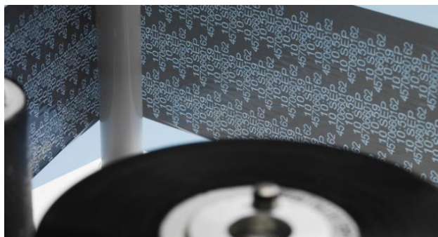
Figuur 27: Thermal transfer lint [67]
