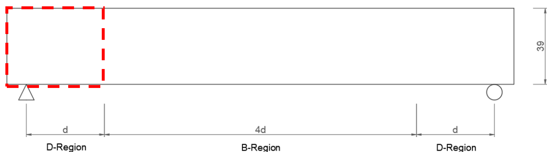
Figure 17 - Step 1: Separate B- and D-regions
