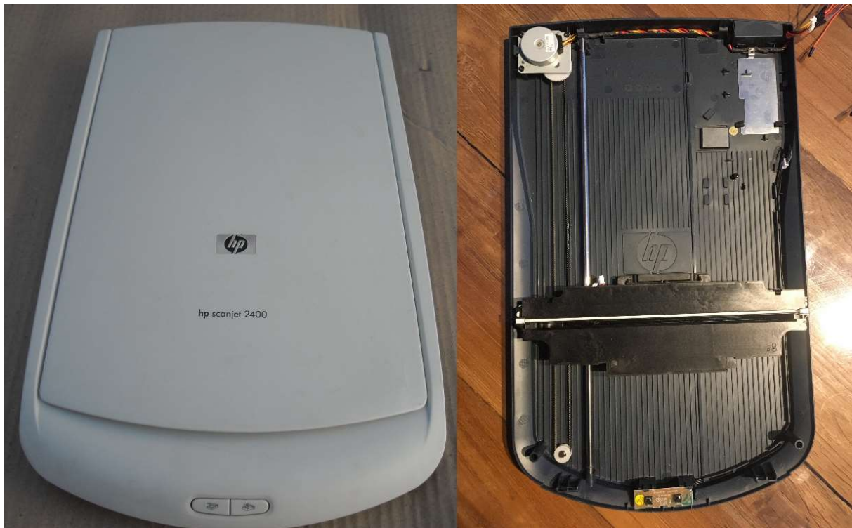
Figure 14: Scanjet 2400 as setup base a) Left side original casing, b) broken apart
