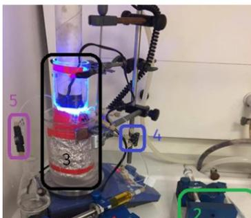
Figure A30. Picture of the microreactor used for the synthesis of the PMMA macroRAFT (picture made by Maarten Rubens). The microreactor is indicated by the black rectangle.
