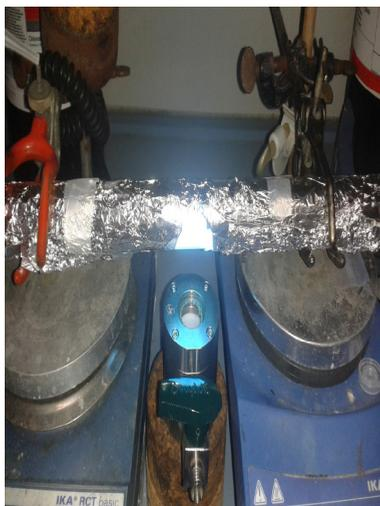
Figure A3. Custom-made chamber with quartz glass window used for surface grafting.
