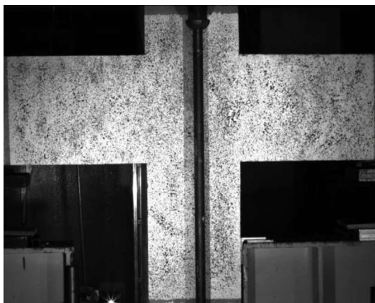
Fig. 7. Surface surveyed by the DIC system.
