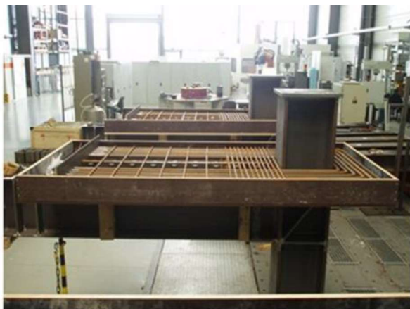
Fig. 2. Test specimens during fabrication.
