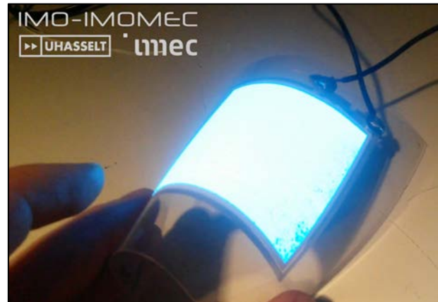
Figure 7: (a) Schematic cross section of the printed electroluminescent device and (b) photograph of a flexed, luminous ACPEL device
