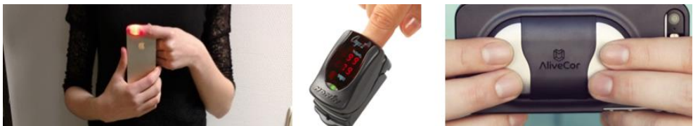
Figure 4: Graphical representation of how measurements are performed using the different devices. Left, FibriCheck application; Middle, Nonin oximeter; Right, AliveCor.
