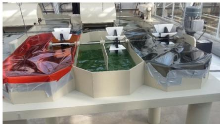
Fig.1 The experimental set-up of the raceway pond reactors in the greenhouse. *Arthrospira* was cultivated under natural conditions in the ponds covered with red and grey light filters and the non-covered pond was used as a control.
