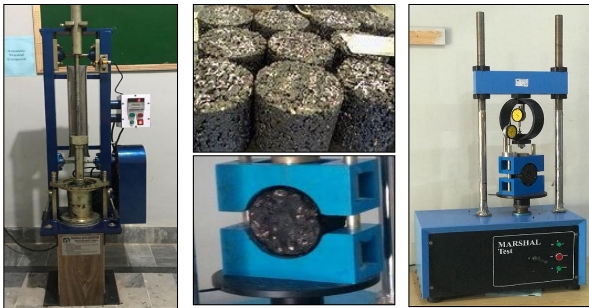
Figure 3. Marshall testing machine with asphalt specimen and compactor apparatus.
