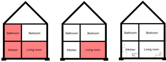
Fig. 5. Three different scales of heating: simultaneous heating of all used rooms (left), multi-zone heating (middle), localized heating (right).
