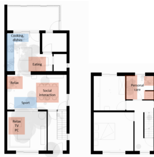
Fig. 6. Potential places to implement localized conditioning systems.
