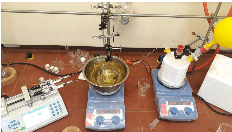
Figure 7: Setup used in the synthesis of monomer mimics. Acryloyl chloride is produced and added immediately to the reaction flask.
