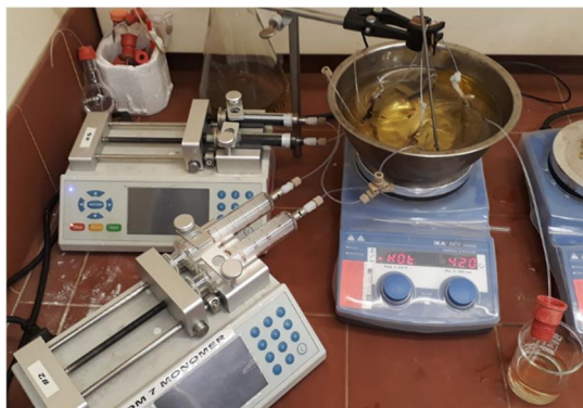
Figure 15: Flow setup for the upscaling of acryloyl chloride production. A replica of the existing reactor was made attached to a second syringe pump. This enables the simultaneous reaction in both reactors doubling the produced amount.
