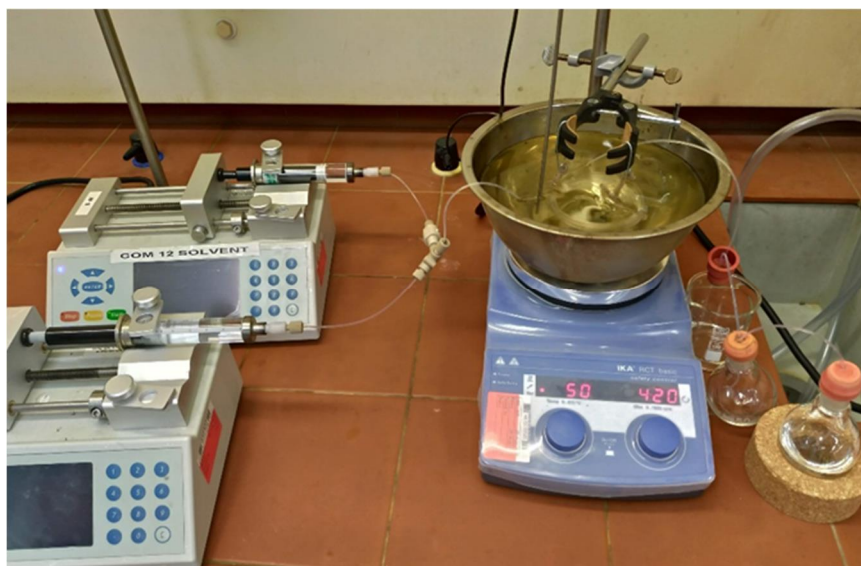
Figure 6: Overview of the experimental setup used for the synthesis of acryloyl chloride.
