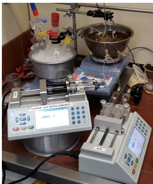
Figure 17: Flow setup for the synthesis of monomer mimics. The produced acryloyl chloride was added dropwise to a vial containing the appropriate amine and TEA in THF.
