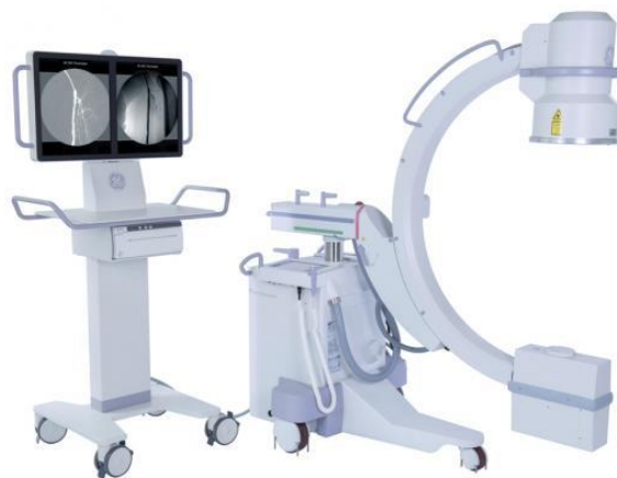
Figure 1: OEC Fluorostar 7900 series C-arm. A mobile C-arm contains an X-ray generator and an X-ray detector in the opposite direction. It can create 2D images from different angles. An additional monitor displays the images in real-time (7). 2D: two-dimensional.
