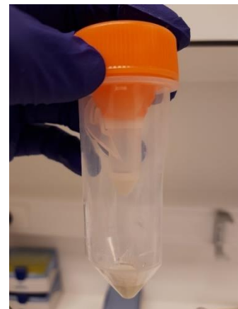
Figure 3 Homogenisation of corpus cavernosum samples with the GentleMACS without any leftovers. The tissue is completely dissolved.
