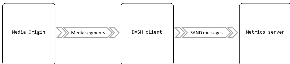
Figure 3.4: An abstract network overview depicting DASH metrics being exchanged via a SAND communication channel between a DASH client and an out-of-band metrics server. The media origin has no knowledge of SAND and does not know that the DASH client exchanges these messages with an external party.
