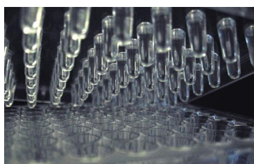
Figure 11: MBEC™ Biofilm Inoculator with 96 well base https://www.genengnews.com/new-products/biofilm-generation/4091
