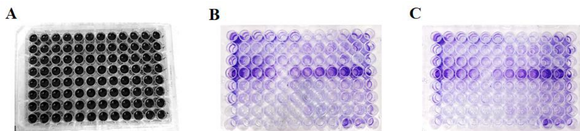
Figure 8: An example of the biofilm assay quantification: (A) Staining of biofilms using 250 \mu L of a 0.1% CV solution, (B) Microtiterplate after rinsing with tap water one time, (C) Microtiterplate after rinsing with tap water three times
