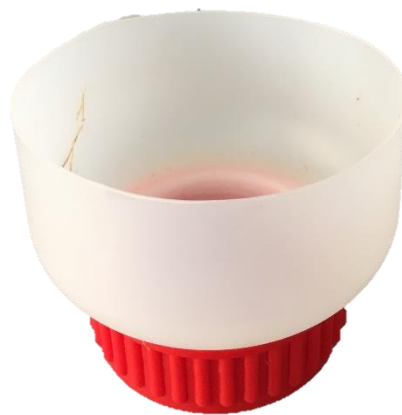
Figure 3.3: Vessel ( \varnothing 6 cm) for the cultivation of the plants that are used to determine the photosynthetic activity. 4 of these vessels are placed in a growth box like the one shown in Figure 3.1 to provide for replicates
