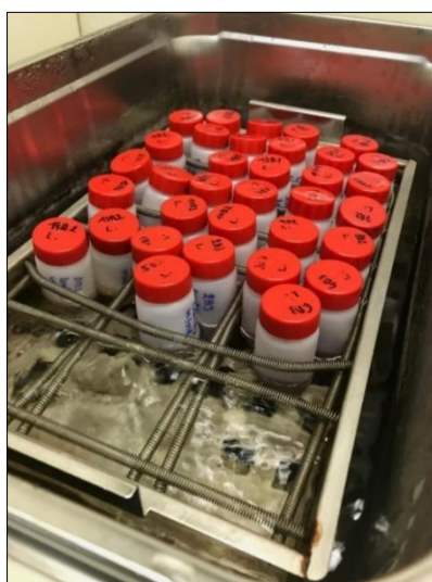
Figure 20: Grant GLS 400 , linear shaking water bath setup
