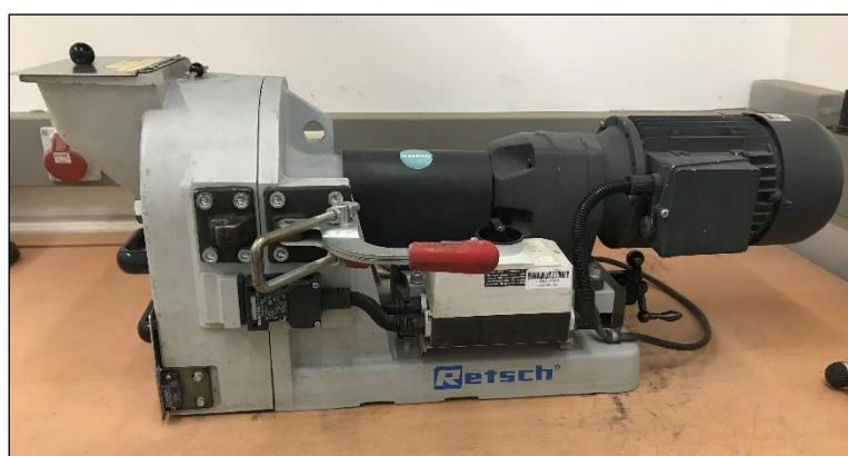
Figure 13: Retsch ® Disc Mill DM 200 , used for grinding the marl
