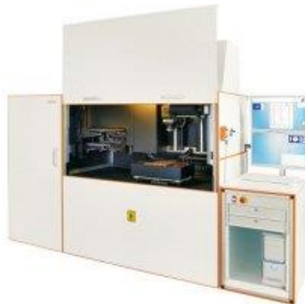
Figure 3.1: LOANA solar cell analysis system [61]
