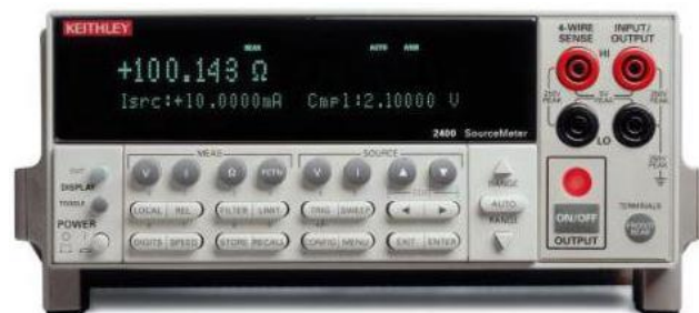
Figure 3.3: Keithley 2400 front interface [65]
