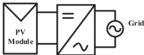
Figure 2.8: Transformer-less inverter [17, p. 1124]
