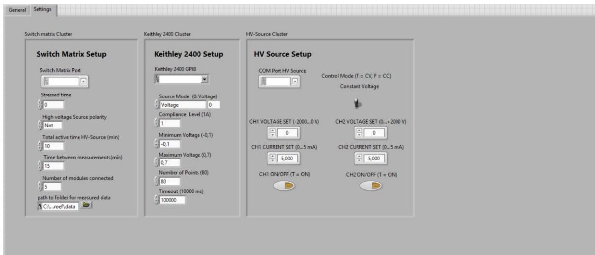
Figure 4.7: Settings tab of the LabVIEW program
