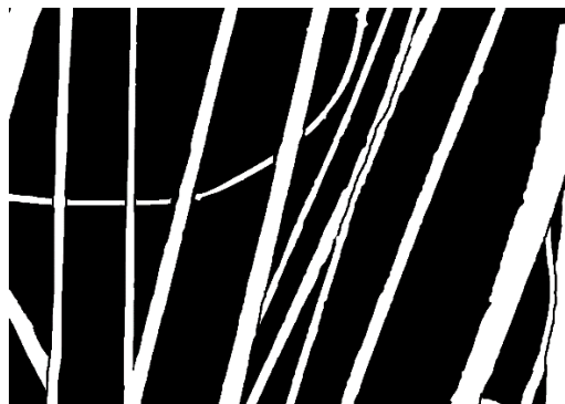
Figure 32: Segmented image generated by the DiameterJ Plugin
