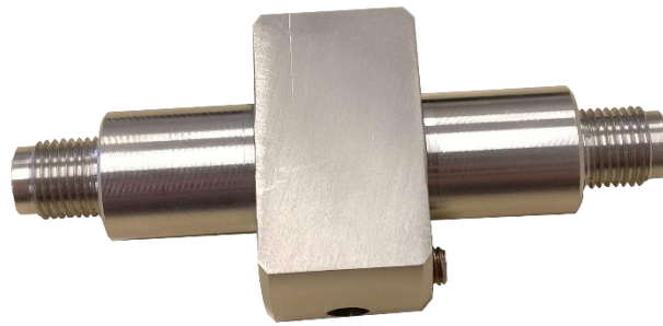
Figure 26: Spinneret design version 2 with threads showing
